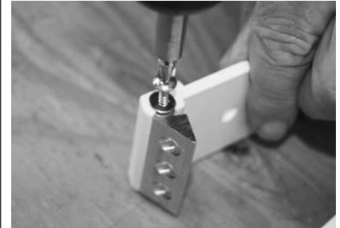
Photo 7C: SECURE LEAF IN PLACE WITH SCREWS
